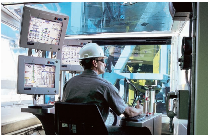
A worker in the control seat of a Helmerich & Payne FlexRig can control drilling, or turn the operation over to an automatic driller.
