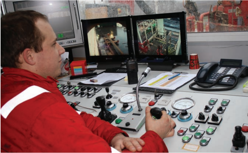
A worker monitors the progress of a well drilled by Shell's automated drilling system.
