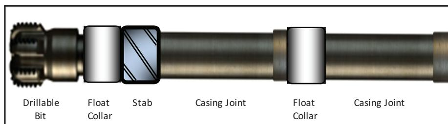
Fig. 1—BHA designed for CwD job in Fields A (as shown) and B (no stab needed and only one float collar, at 13 m from bit).
