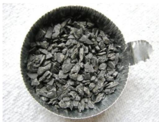
**Fig. 1—After shale erosion test in customized WBM.**
