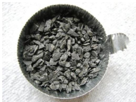
**Fig. 1—After shale erosion test in customized WBM.**
