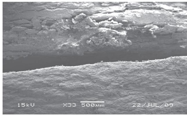
Fig. 4—Fayetteville/Morrow Shale after 24-hour soak in fresh water.
