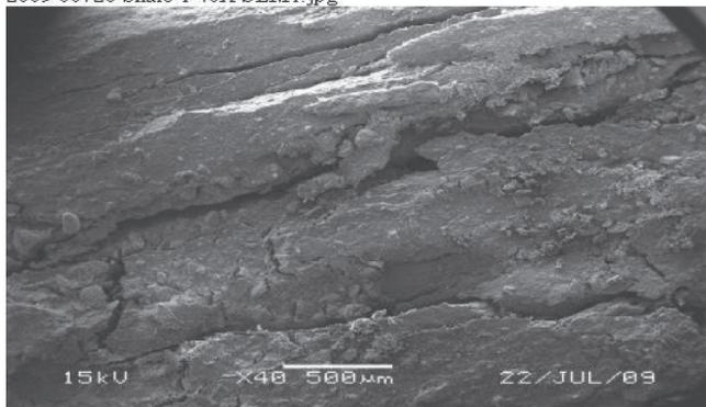
Fig. 5—Fayetteville/Morrow Shale after 24-hour soak in typical inhibitive WBM.
