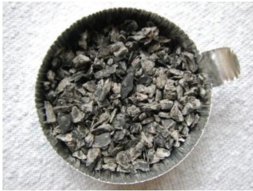
Fig. 2—After shale erosion test in OBM.
