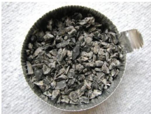
Fig. 2—After shale erosion test in OBM.
