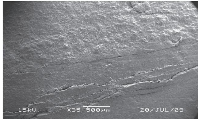
Fig. 6—Fayetteville/Morrow Shale after 24-hour soak in customized WBM for Fayetteville shale.
