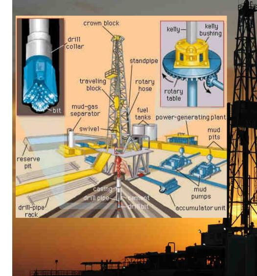
**Drilling Fluid** is circulated by being pumped down the **drill string**
