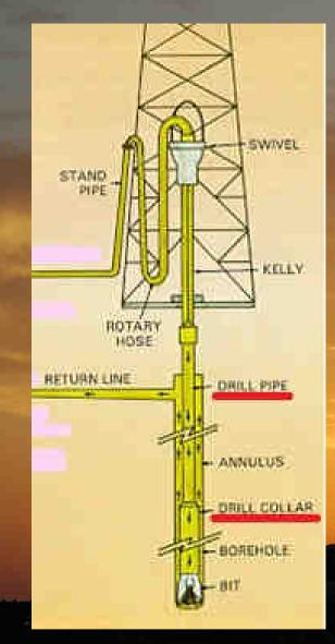
The **drill string** is the mechanical assemblage **connection** the rotary drive on **surface** to the drilling **bit on bottom** of the hole
