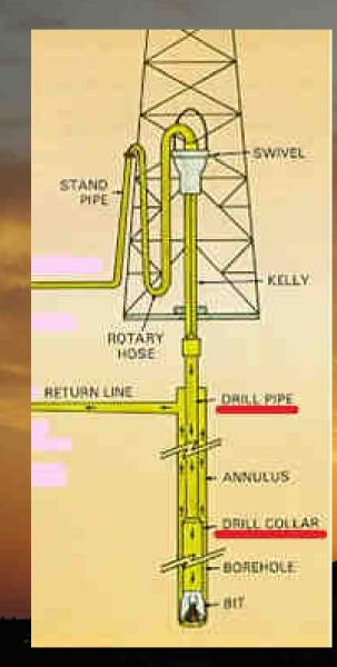
The drill string is the mechanical assemblage connection the rotary drive on surface to the drilling bit on bottom of the hole
