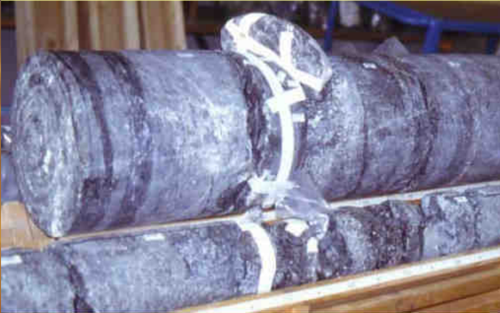
Core from KTB Pilot Hole
