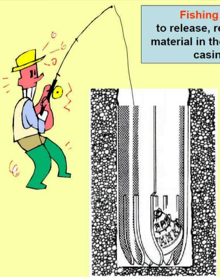
Fishing is any operation or procedure to release, remove or recover tubulars or other material in the hole that adversely affects drilling casing or completing operations
