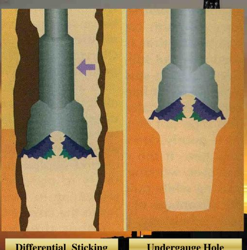
Differential Sticking Mud Cake Too Thick Undergauge Hole Worn Bit Gauge
