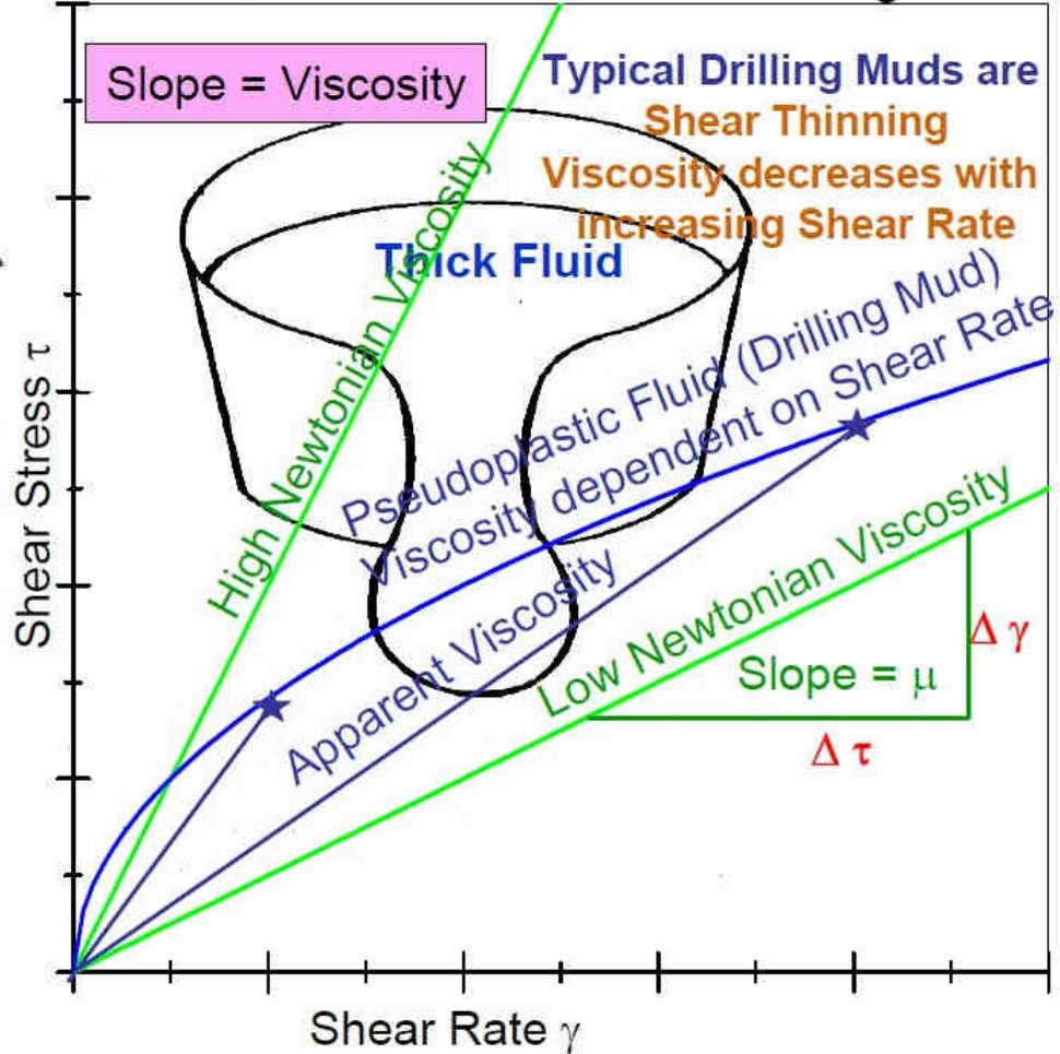
Typical Drilling Muds are Shear Thinning
