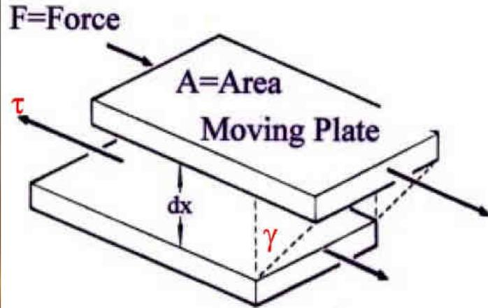
Shear Rate  $\gamma = dv/dx$
