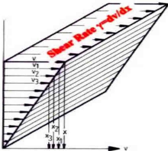
Shear Stress - Shear Rate Diagram
