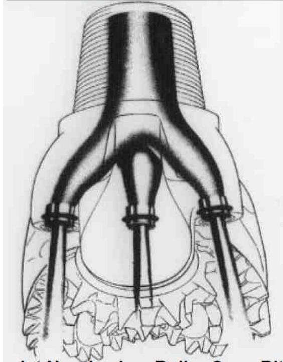
Jet Nozzles in a Roller Cone Bit
