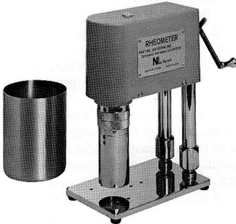
Determination of **Shear Dependent Viscosity** by Measuring **Flow Curve** at different Rotational Speeds
