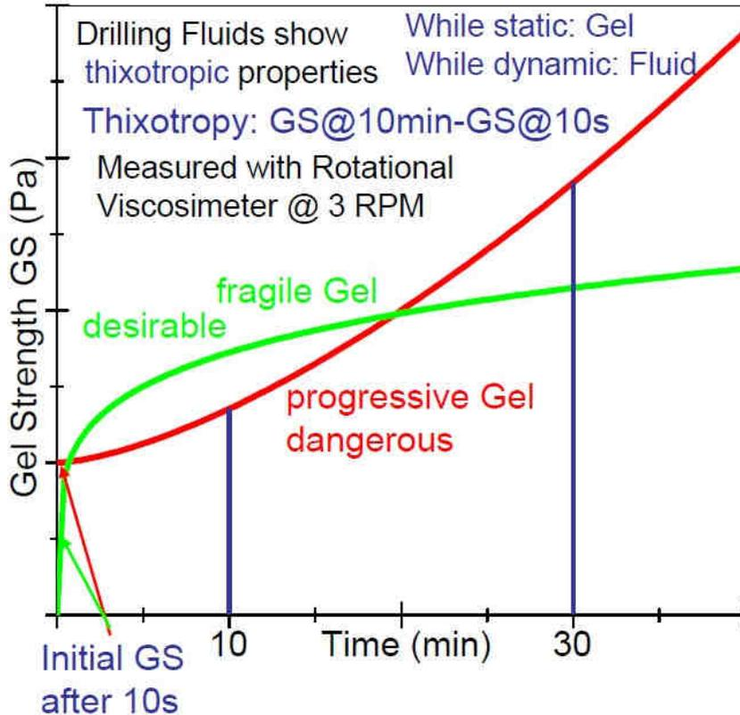
Pump Pressure necessary for Breaking Gel
