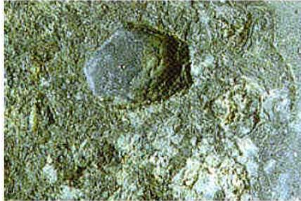
Stress Corrosion at DP-Tooljoint
