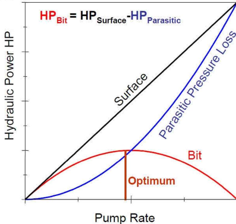
Impact Parameters on Parasitic PL
